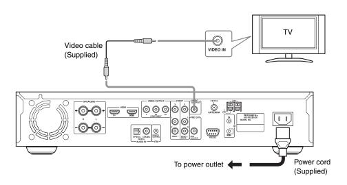
This receiver is equipped with copy protection technology. Do not connect this receiver to your TV via a VCR using Video cable, as the picture from this receiver will not appear properly on your TV. (This receiver may also not be compatible with some combination TV/VCRs for the same reason; refer to the manufacturer for more information.)
